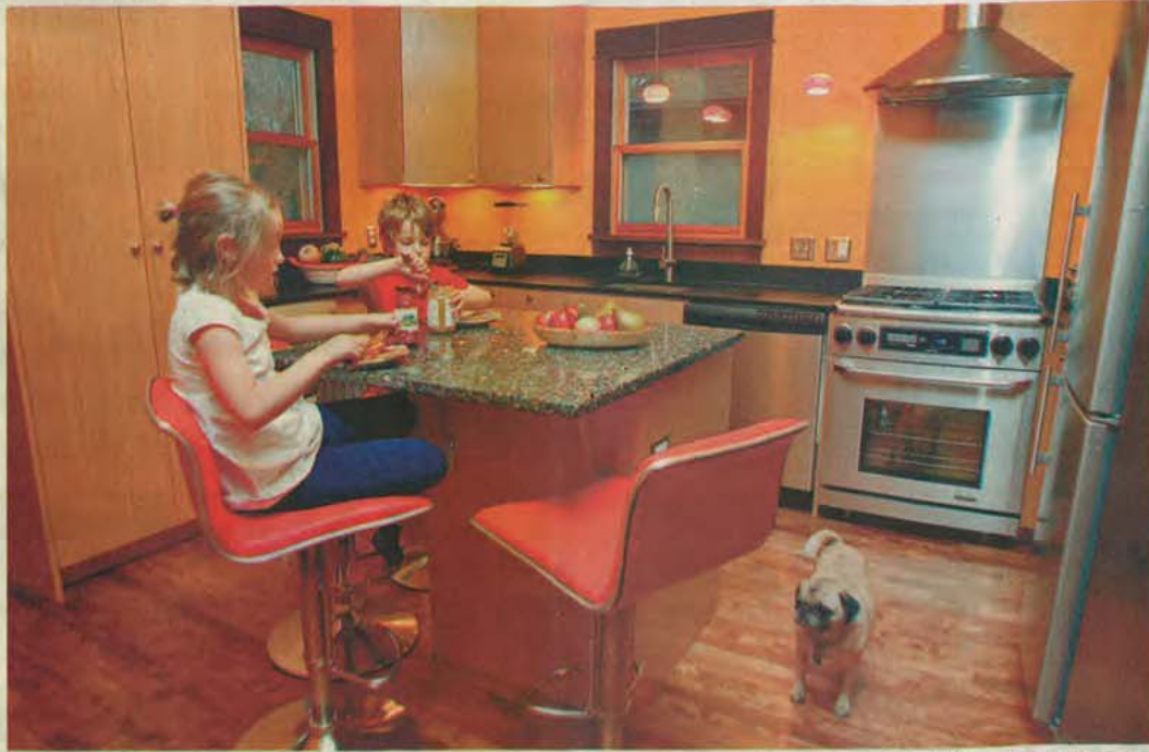
Nora and Eli Hatting have a snack on the recycled-glass-topped center island in their eco-friendly kitchen. Formaldehyde-free cabinets and low-VOC paints and finishes were also used.
